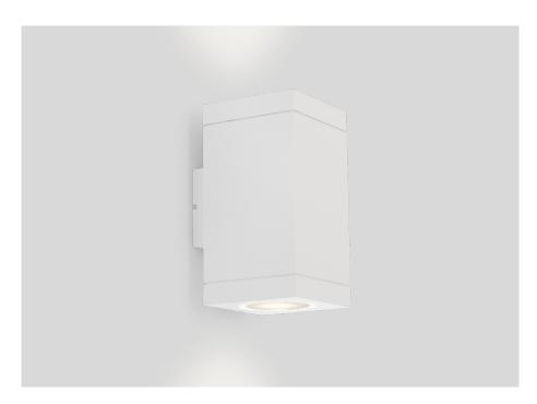
Rectangular wall surface luminaire made from aluminium; surface White Matt; powder coated; matt texture; RAL 9003; lamp socket GU10; lamp type PAR16; 2x max. 5W; 100 - 240 V; up and down light emission; degree of protection IP65; PC1; lamp not included;
