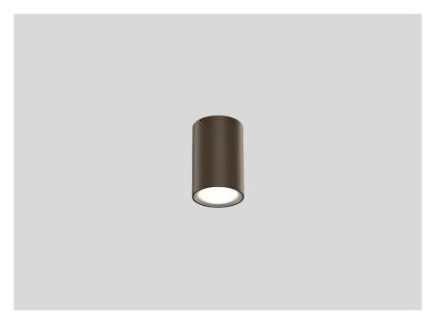
Cylindrical ceiling surface mounted downlight made from die-cast aluminium; surface Bronze; wet painted; brushed; with COB (Chip on Board) technology for maximum efficiency; phase-cut dim; light colour 3000 K; CRI  $\,$  90; 220 - 240 V; degree of protection IP65; PC1; light source not replaceable;
