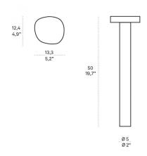
Floor lamps with a dark grey or corten painted die-cast aluminium frame and a satin-finish opaline polycarbonate diffuser. The high IP rating (IP54) makes the lamps ideal for indoor and outdoor use.
